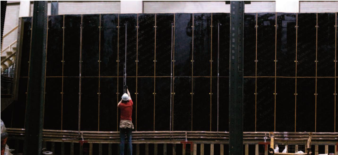
As part of research on the shear strength of very thick one-way slabs, we have constructed a reinforced concrete “slab strip” specimen four metres in overall depth and about 20 metres long.
