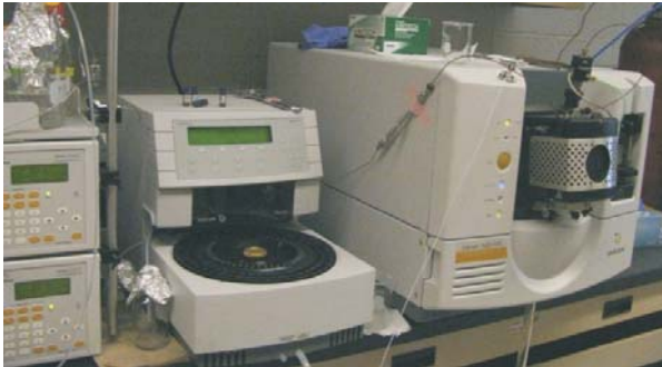
Figure 1: Liquid chromatography-mass spectrometry (LC-MS) at University of Toronto Drinking Water Research Lab used for detection and identification of chemicals in water samples
