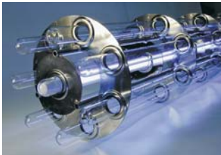
Figure 2: UV reactor (source: www.awwa.org)
