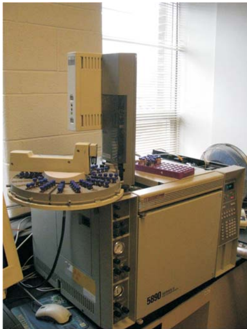
Figure 1: Hewlett Packard 5890 Series II Plus Gas Chromatograph (Mississauga, ON) using an electroncapture detector (GC-ECD) and a DB 5.625 capillary column
