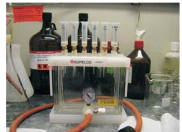
Figure 2: - Vacuum manifold for solid phase extraction of MX in water
