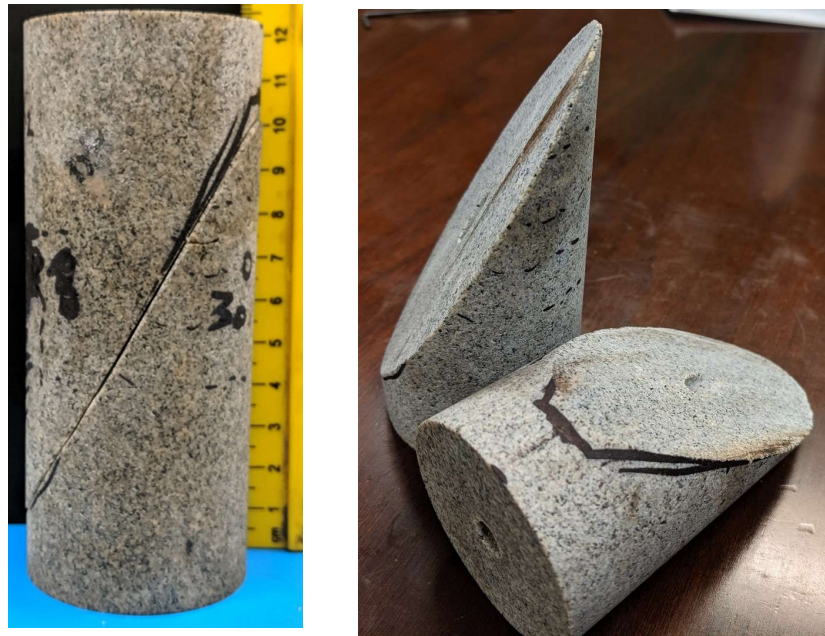
Figure 1. Shows the saw cut Westerly granite with a central Fluid-injection hole to access the fault plane
